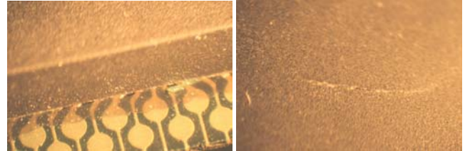
Image 0: Left image – side shot of BGA with crack between the plastic cover and the BGA substrate. Right image – crack on top surface of plastic BGA.
