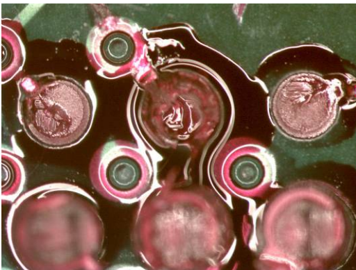
Figure 17B Dye & Pry Image PCB Side (pin A26, board 17159)
