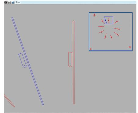
**Figure 5:** A CAD drawing that was automatically generated through the programming process. Interactive tools permit slight modifications of tool position. Copy/paste functionality is very useful for repeating patterns.
