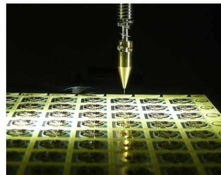
**Figure 1:** MEMS devices set up for an automatic non-destructive wire pull test.
