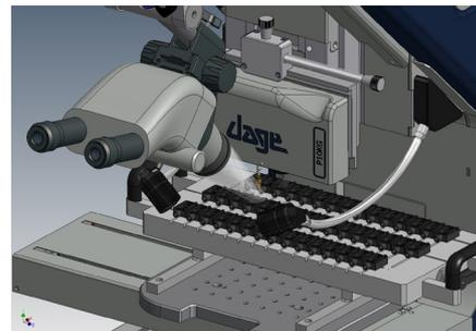
**Figure 2:** Sample holder designed for automatic bond testing of individual MEMS devices loaded into the system.
